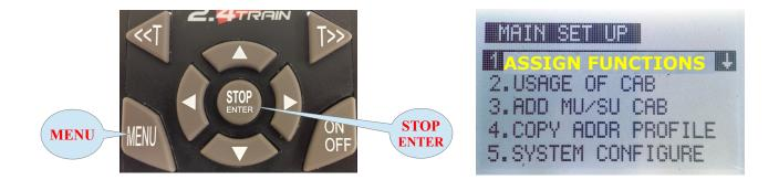
Under '1.ASSIGN FUNCTION' choose your 'LINK /BIND ADDRESS (49)'. It's recommended to start with (**00**) as your first link address. To quickly get to link address (00) press the 'STOP/ENTER' BUTTON. Press the bottom arrow to select Rx-Type then press the right arrow to select 'BASE RX'
