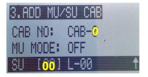
The linking process is finished press the Menu button twice to get back to the main screen. At the bottom of the main screen it should show up 'LINK OK'.
