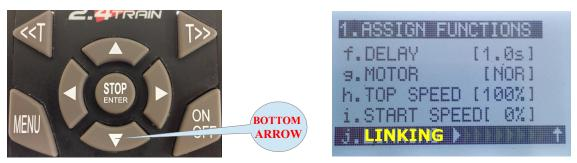
Press the Red Push button cord on the receiver or you can press the Red button directly at the corner of the receiver and the Blue LED on the receiver will flash brightly indicating the linking process has started. Release the button as soon as the Blue light starts to flash. Press the **Stop/Enter** button on the transmitter and the transmitter should indicate linking Passed.
