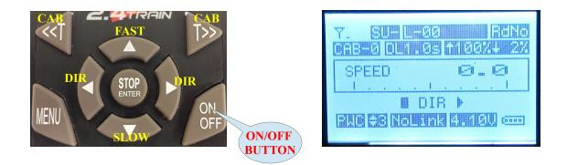
Press the MENU button on the transmitter and select '1. ASSIGN FUNCTIONS'. To select this function press STOP/ENTER button on the transmitter.
