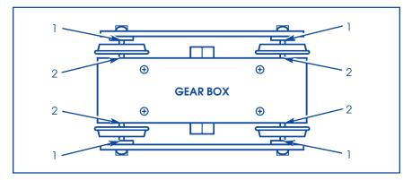
**1. SIDEFRAME JOURNAL BOX:** The axle ends fit into brass bushings which bring power into the locomotive. These brass bushings should periodically be cleaned out and lubricated with a small amount of USA Trains electrically conductive lubricant (USA Trains Part #R50002). Use only our conductive lubricant to avoid loss of electrical contact which could cause your locomotive to lose power or run erratically. The frequency of lubrication depends on your operating conditions.
