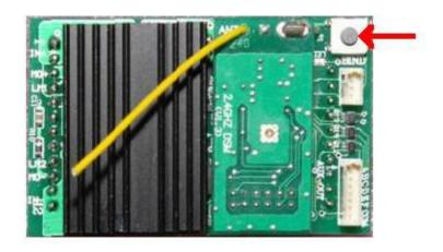
When you push on the cord or the black push button the red LED on the receiver (and locomotive headlights if connected) will flash brightly indicating the linking process has started. You need to press the Stop/Enter key and a few seconds later the transmitter should indicate linking passed.
