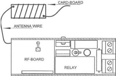
Use a rubber band to hold the antenna wire in place to the end section of the model. This prevents the antenna from touching any metal parts.
