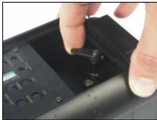
fig. #19 Opening the butane valve
