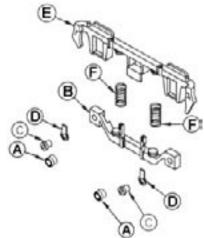
\*Example of ART-29109 passenger truck application or trucks with electrical pick up. Other passenger trucks may differ.
